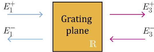
Figure 4. Propagation in one dimension from an incoming and outgoing plane wave on a grating plane, related to the transfer matrix \mathbb{R} .
