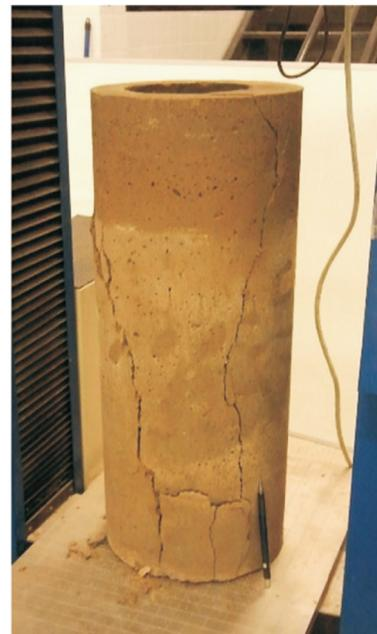
**Figure 22** - Sample after failure stage (laboratory test).
