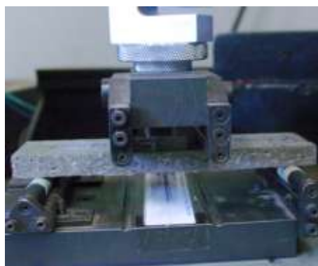
FIGURE 1. Four-point bending device with a specimen and load cell.
