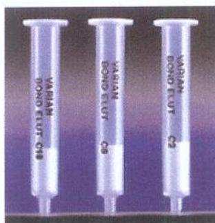
**Figura 14:** coluna de sílica Bond Elut Jr (Varian®).
