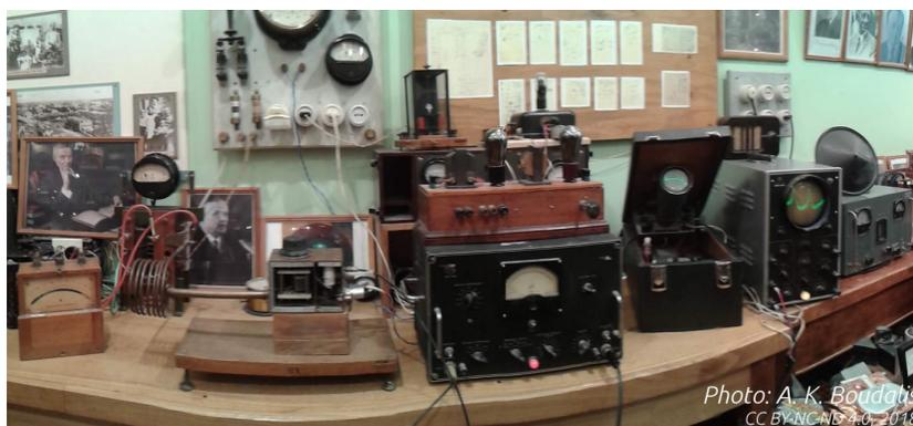
Figure B.1: Photograph of Zavoisky's experimental setup for the first ESR experiments ever performed. Figure taken from [91].
