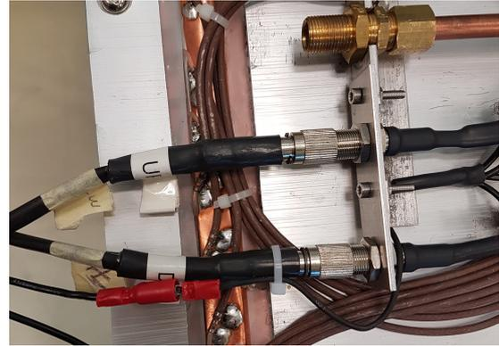
**Figure 4.18:** Left: Proposed adapter the chamber patch panel which make it possible to replace a tripolar by a jupiter HV connector. Right: Try out of the proposed HV connector replacement.
