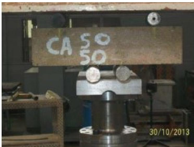
Figure 6 Applied Equipment to the dynamic tensile traction flexural test
