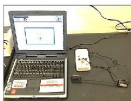
Figure 2. Electrogoniometer with two sensors connected by an optical fiber, that are positioned as shown in Figure 1 and also connected to a computer.
