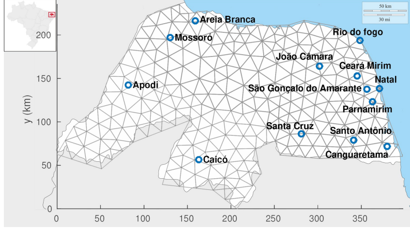
Figure 8 – Linear finite element mesh approximating Rio Grande do Norte state. Circles represent cities with relevant incidence data.
