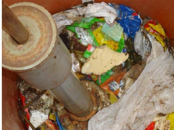
Figure 2 - Compression process inside the permeameter.
