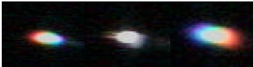
**Figure 7:** Image projected in a screen of an halogene lamp passing through the critical point.
