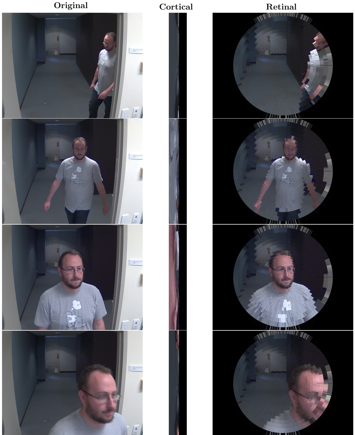
Figure B.1: Examples of images reconstructed with a log-polar mapping. Left-column images are the original ones. Middle-column images are the cortical versions after a log-polar mapping procedure. Right-column images are the retinal images after an inverse log-polar mapping procedure has been performed on their cortical versions. The original images come from the ChokePoint Dataset [105].
