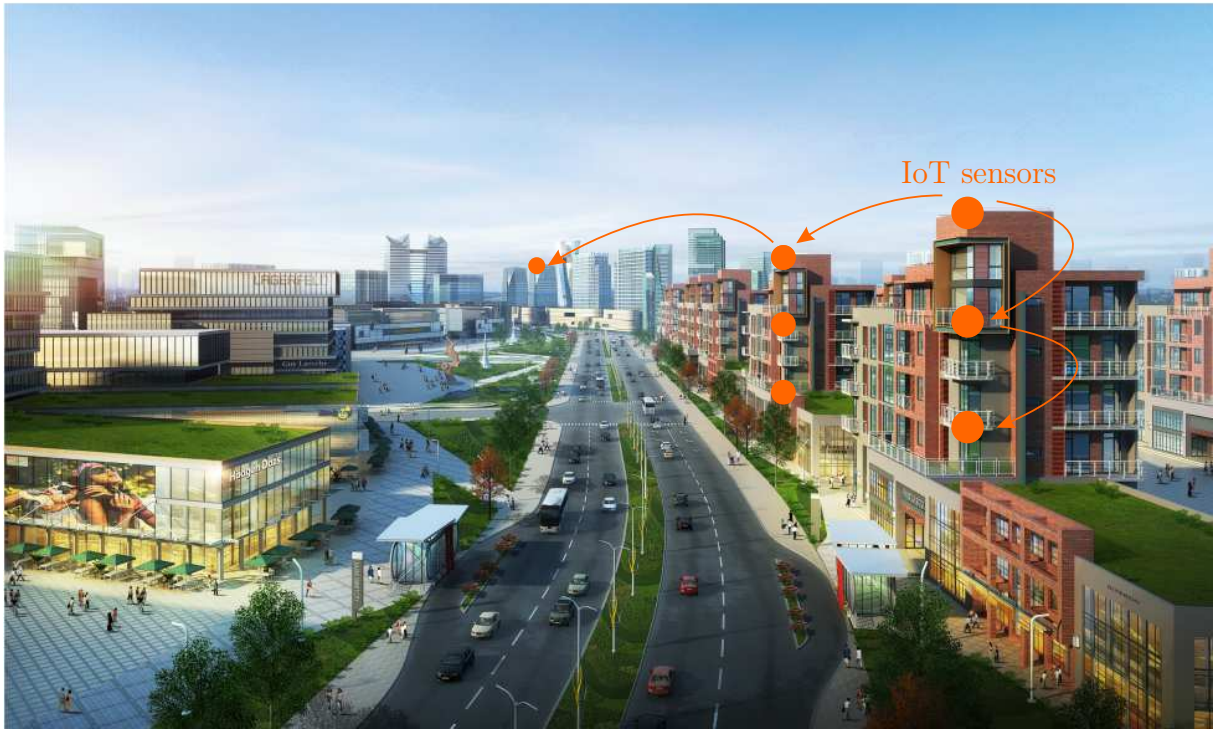
Figure 2.2: Sensor communication in smart structures in the context of smart cities. Smart buildings and smart structures contain sensors connected in a network, which communicate the building state at relevant intervals and may provide information about the building's movement in response to strong winds or earthquakes and about the structural health, temperature, vibration, and displacement. If any problem is encountered by the processing of these data, actuators in the building can absorb shocks or reduce its movements and a warning can be sent to other buildings or structures so that the people responsible for them take the necessary actions [98] (modified).
