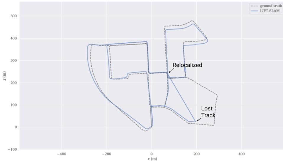
Figure 5.5: Example of trajectory when relocalization is performed, after losing the track the camera is relocalized after finding a revisited place.
