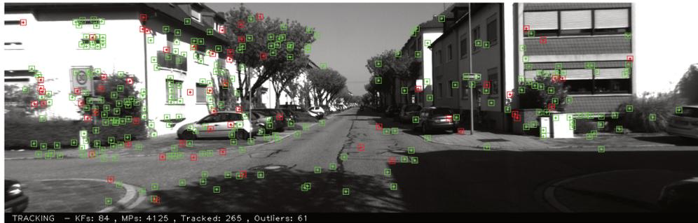
Figure 5.3: Keypoints and Outliers in feature tracking performed in KITTI dataset, green squares are the projected LIFT keypoints that were considered inliers and the red squares are the outliers.
