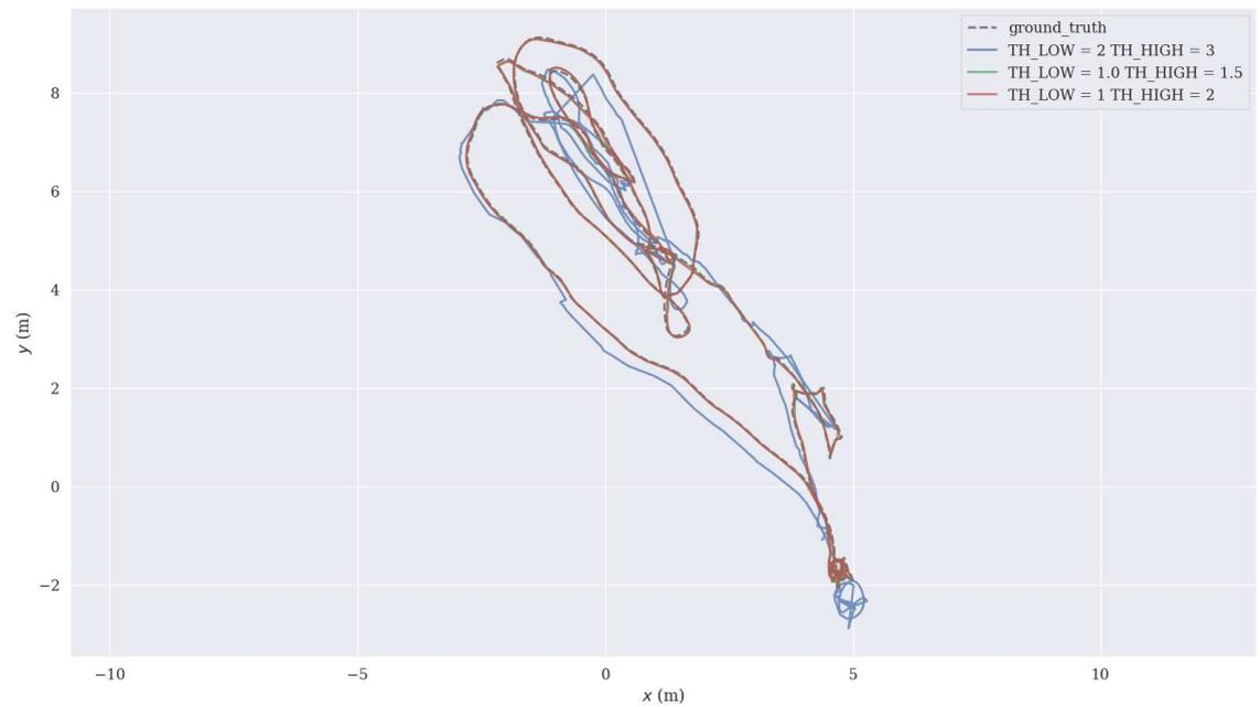
(b) Comparison of LIFT-SLAM performance with different matching thresholds in EuRoC *MH\_01* sequence.
