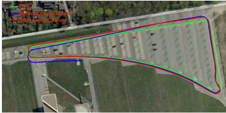
Figure 2.1: Comparison between SLAM and odometry on a self-driving car trajectory. The ground-truth positions are provided by a GPS are in the green line. The blue line shows the path estimated by odometry. The red line shows the global path estimated by SLAM, performing loop-closure to improve previous positions. Adapted from [45].
