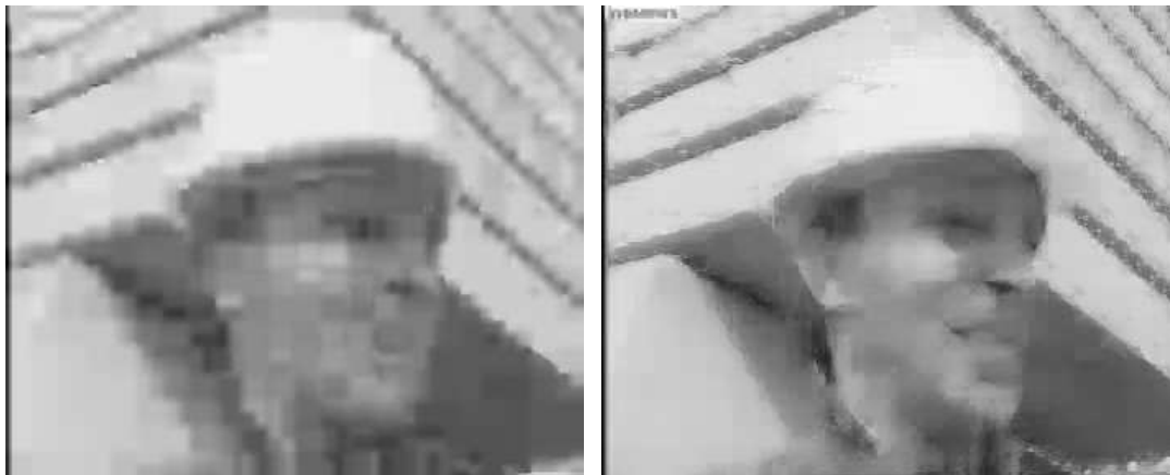
(a) A frame from the 'Foreman' sequence encoded by x264 (b) The same frame encoded by the proposed method
