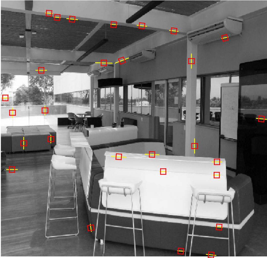
Figure 3.8: Example of the lines that were detected and passed all criteria along with their ROIs.
