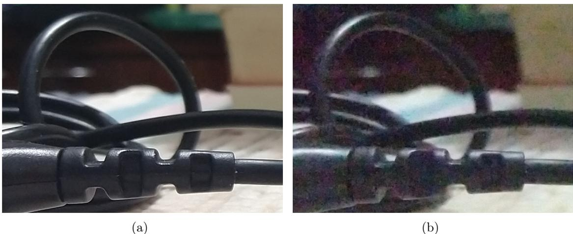
Figure 2.3: Effect of ISO speed (ISO 12232) in the perceptible noise. (a) ISO speed = 100; (b) ISO speed = 3197.
