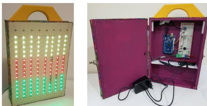
**Figure D. 1** To the left, SAMLight in use. To the right, SAMLight's internal circuits.
