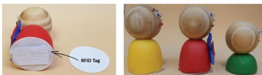
**Figure 8.4.** To the left, RFID labels placed on the base of each TangiSAMM manikin and its Braille symbol. To the right, TangiSAMM manikins - side view.
