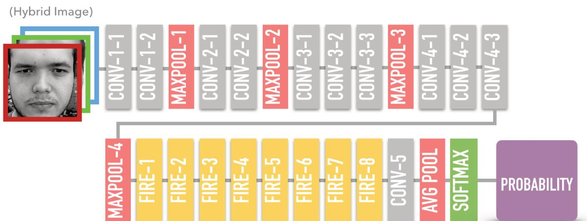
Figure 4.6: HFCNN architecture outline. Each convolutional layer (gray boxes) are followed by ReLU operations and each Fire module (yellow boxes) have the internal configuration depicted by Fig. 4.5.
