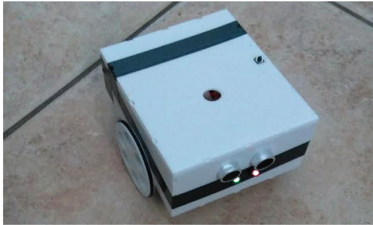
Figure 3.7: Robot used in our experiments. The robot has two motor encoders, a Bluetooth adapter, an ultrasonic sensor, two LEDs and a button. It also has a hole children can put a pen in to use the robot for drawing.
