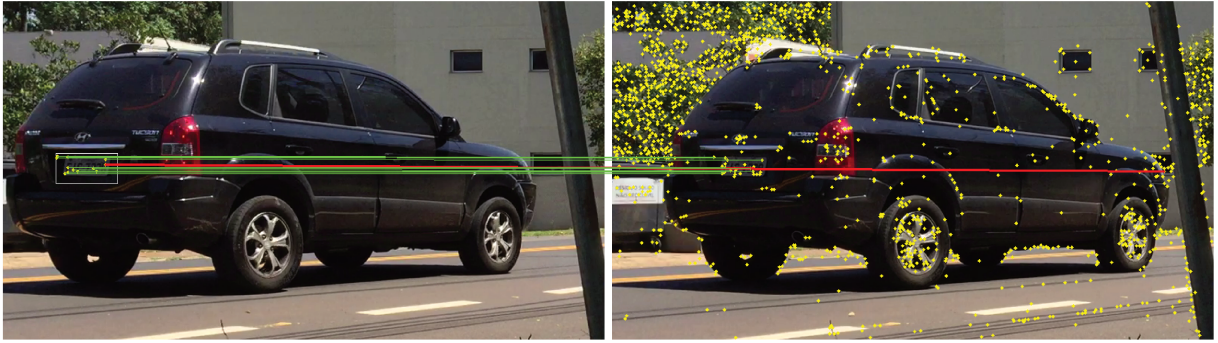
Figure 5.11: Tracking using SIFT. The white polygon is the region around the license plate in F_k . Yellow dots are the SIFT keypoints inside the small region in F_k and in the entire image F_{k+1} . Green lines are matches between the frames. The red line is an incorrect match that will not be used.
