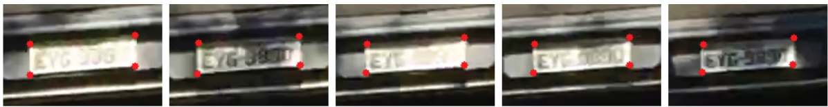
Figure 6.5: Cast shadows may impact the tracking step. The red dots show that PyrLK and PyrDense could track the frames even with a different lighting condition in each consecutive frame.
