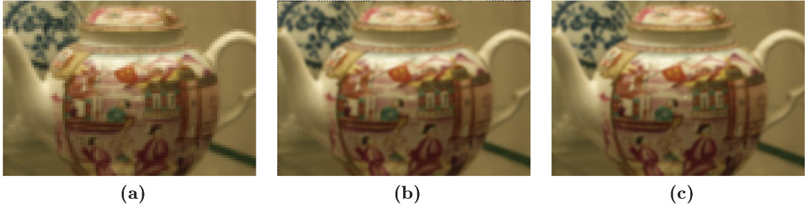
Figure 3.13: In (a), an LR image is zoomed in by a factor of four using Nearest Neighbors interpolation. In (b), 35 LR images are super resolved by ISR_1 . In (c), the blurred image that generated the LR observations in the pool.
