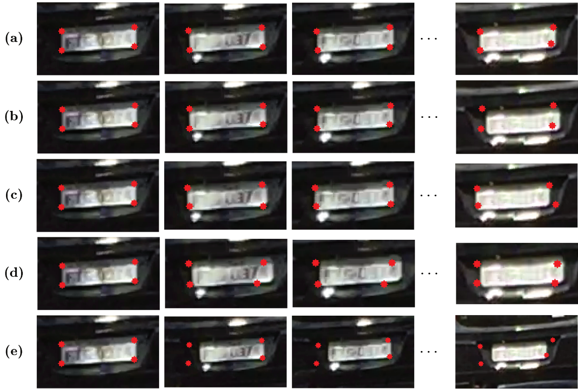
Figure 6.6: Examples of an input video tracked by PyrLK (a), PyrDense (b), SIFT (c), SURF (d) and ORB (e).
