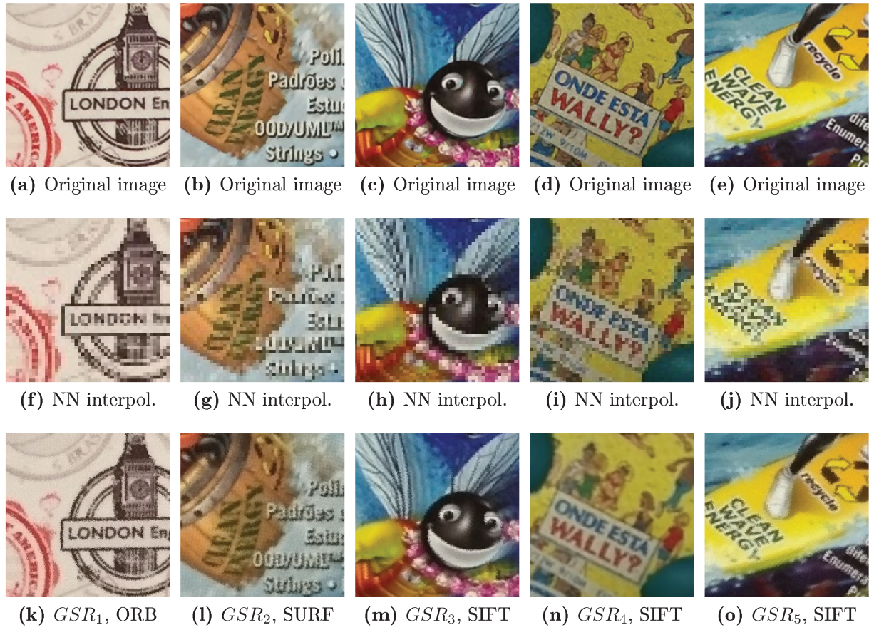
Figure 4.39: LR versions of 25 real images taken by a mobile phone generate a 4\times higher image. In the first row, the original target images H_k for different scenes. In the second row, each L_k is zoomed in by a factor of four. In the last row, the super-resolved image I_{SR} using different variations of GSR , and different registration methods. Unlike Experiment #1 , the LR images differ from each other by perspective transformations in this setup, and not only by rotations and translations.
