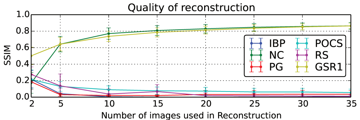
Figure A.5: Quality of different reconstruction algorithms as a function of the number of LR input images.
