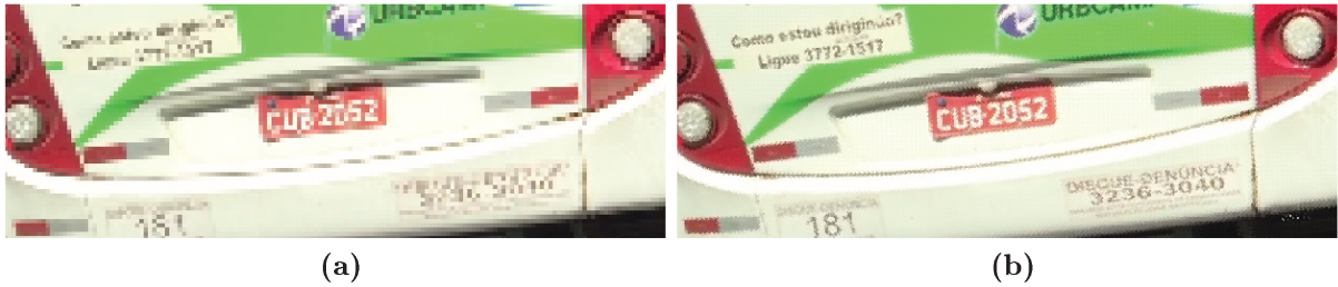
Figure 5.1: Super resolution vs. interpolation: (a) Piece of a low-resolution video frame ( 384 \times 216 pixels) of a moving bus in a real-world traffic video, zoomed by a factor of four using a simple nearest-neighbor interpolation; and (b) Super-resolution version of the same piece, using eight consecutive input frames of a video. Not only the license-plate alphanumerics, but also other characters over the outer surface of the bus, are visually easier to identify in (a) than in (b).
