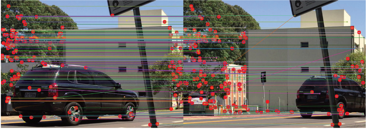
Figure 5.2: Matches between pairs of keypoints found by SIFT.
