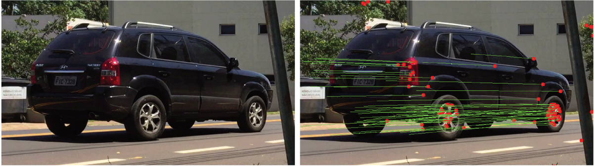
Figure 5.9: PyrLK feature tracker to estimate the optical flow.
