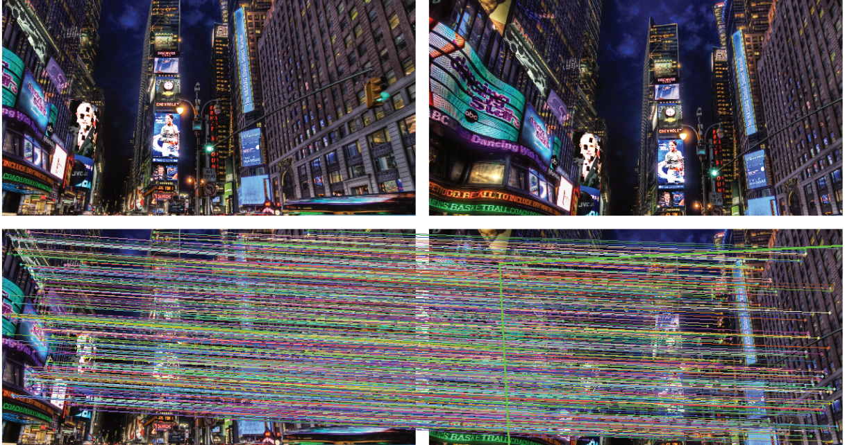
Figure 4.6: Matches between two LR images using SIFT.
