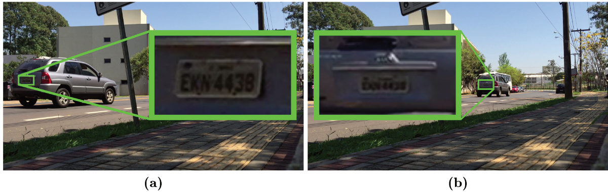
Figure 6.1: The license-plate alphanumerics are easily readable in the first video frames (a) but not in the last ones (b). The first frames are used to create the ground-truth files, and the last frames are used to be reconstructed and recognized. The same zoom-in factor was applied to the license plates in (a) and (b).
