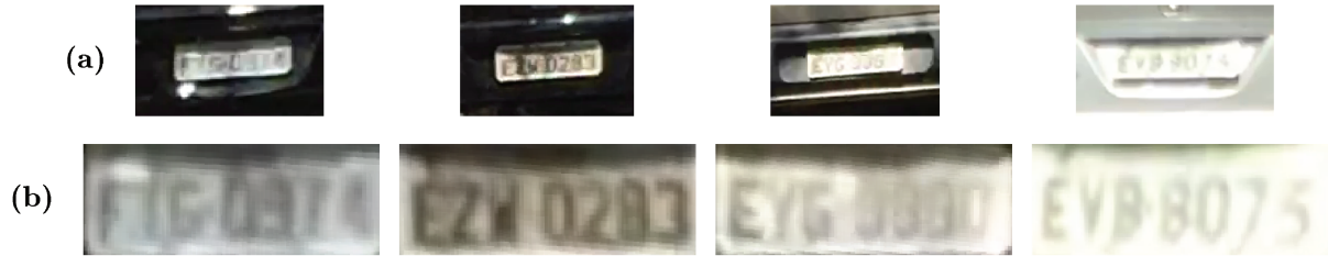
Figure 6.2: Output examples of the proposed framework. In (a), single frames with low-quality resolution. In (b), five consecutive frames are combined into a super-resolved image, richer in details.
