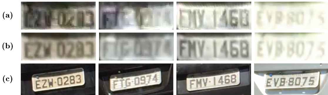
Figure 6.10: Quality of the reconstruction applied to frames with illumination and shadow issues. In (a), the initial frame without super resolution. Then, the results for GSR_4 (b). In (c), a frame with a good resolution of the license plate.
