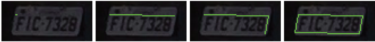
Figure 5.6: User choosing four points and creating a bounding box around the license plate of interest.
