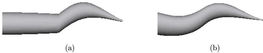
Figure 10.1: A comparison between space deformations (a) without and (b) with C^1 continuity.
