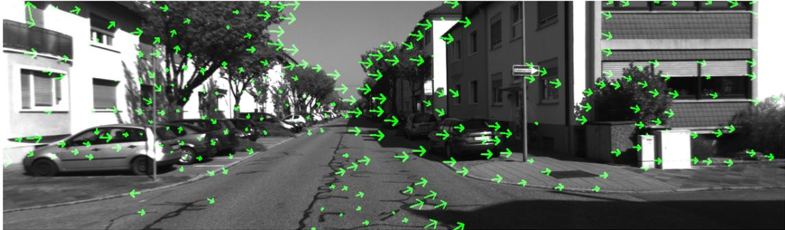
(a) Optical flow during a rotational motion.
