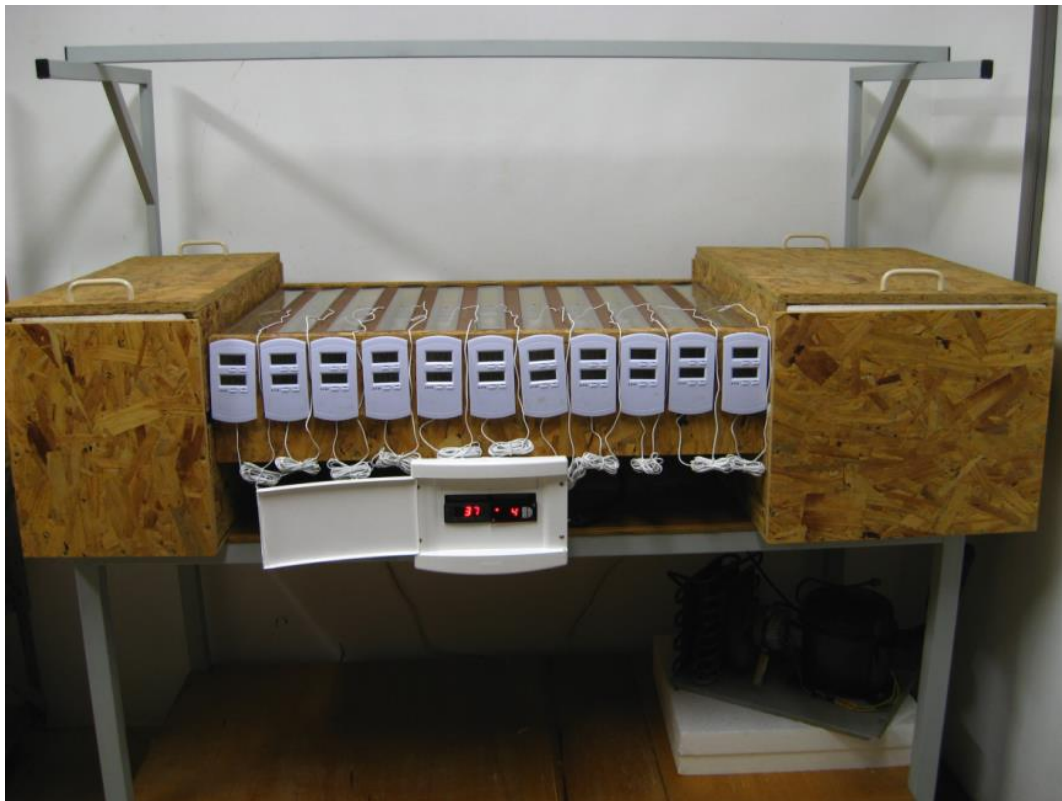
Figure S1. Fogleman's apparatus used to produce the thermal gradient with eleven different temperatures to describe the reaction norms of Drosophila mediopunctata .
