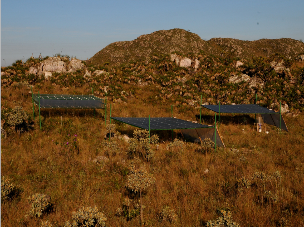
Figure 1. Study area: vegetation of campos rupestres at Serra da Canastra National Park. Plots with closed roofs represent the drought treatment and the plots with open roofs represent the control treatment.
