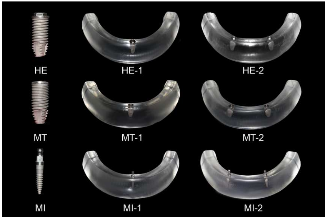
Figure 2. Implants (EH, MT, MI) and photoelastic models (EH-1, MT-1, MI-1, EH-2, MT-2, MI-2) designed for each group. EH, external hexagon. MT, Morse taper. MI, dental mini-implant. EH-1/-2, external hexagon model with 1/2 implants. MT-1/-2, Morse taper model with 1/2 implants. MI-1/-2, dental mini-implant model with 1/2 implants.
