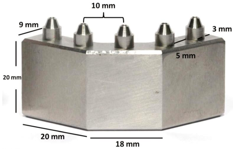
**Figure 1.** Stainless steel master model and disposition of the abutment analogs.
