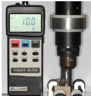
**Figure 3.** Digital torque meter coupled to the device.
