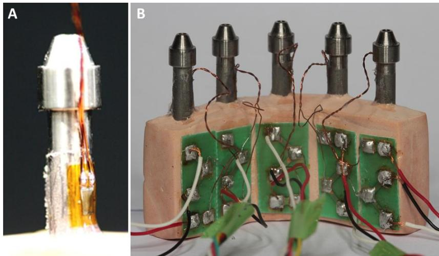
**Figure 4.** A) Closer view of the strain gauge bonded; B) Strain gauge model with a quarter Wheatstone bridge.
