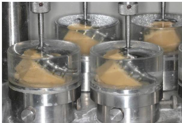
**Figure 2.** Frameworks positioned for cyclic loading.
