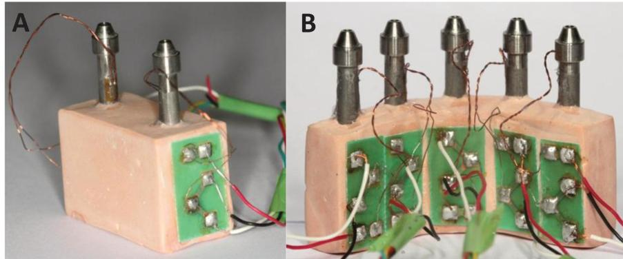
**Figure 3.** Strain gauges bonded on analogs surface with a quarter Wheatstone bridge. A) FPD; B) FFP.
