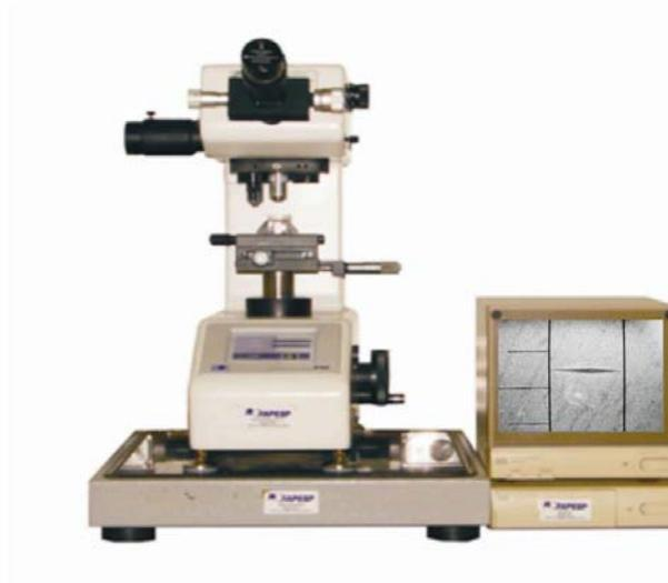
**Figura 4.7** – Microdurômetro Microhardness Tester, Future Tech FM-1E.
