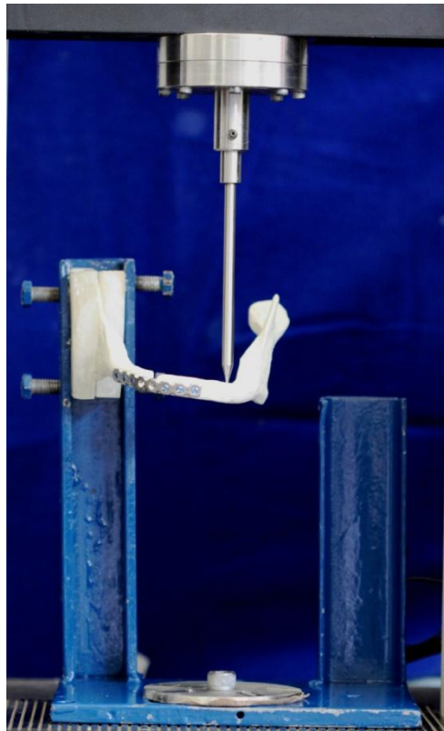
Figure 2 – Custom made test platform with rigid stabilized right condyle, allowing free movement of the distal segment by flextorsional loading forces.
