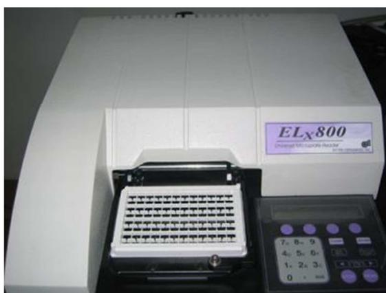
**Figura 8:** Leitor de Microplaca Bio-Tek Instruments, ELX 800
