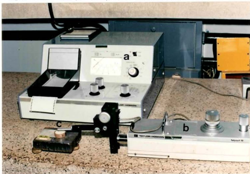
Figura 4 - Rugosímetro Talysurf 10 Taylor-Hobson
