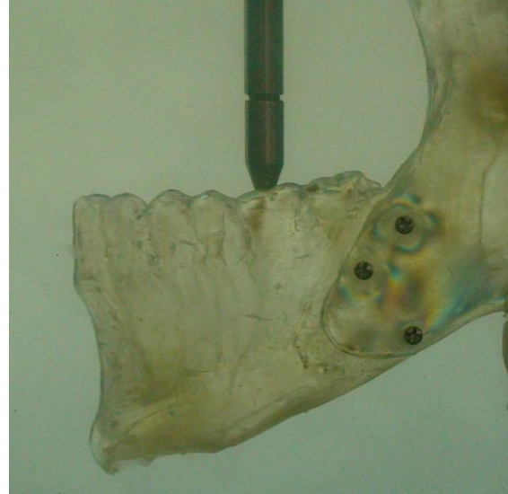
Figure 6 – Photoelastic test of the Reversed L arrangement fixation
