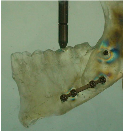
Figure 5 – Photoelastic test of the Hybrid fixation technique
