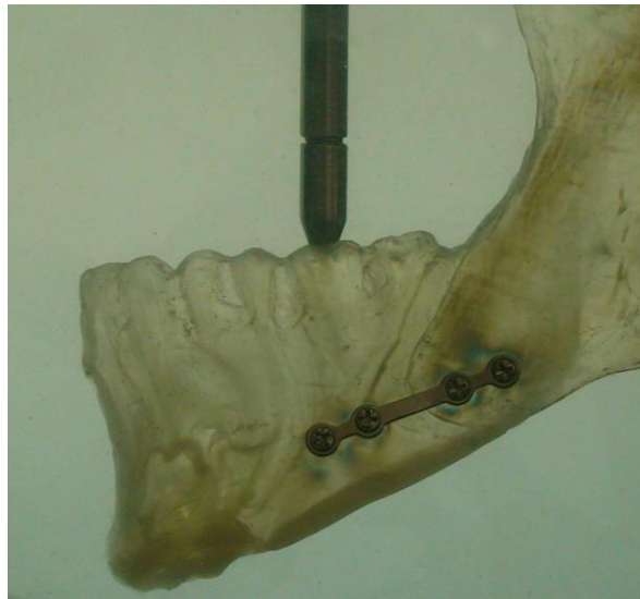
Figure 7 – Photoelastic test of the Miniplates and screws fixation
