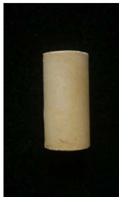
Figure 2 - Sample used for the testing of compressive strength
