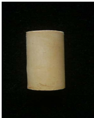
Figure 2 - Sample used in the testing of compressive strength
