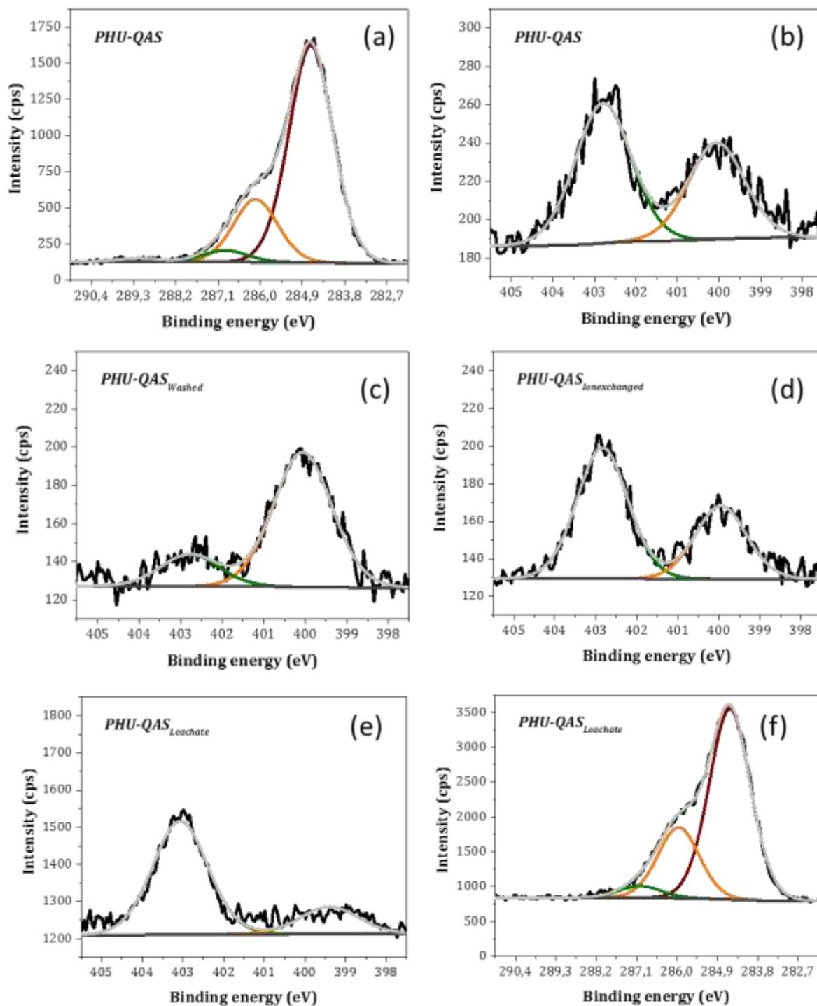
**Figure 5.** XPS narrow scans for: **a)**  $C_{1s}$  for PHU-QAS coating; **b)**  $C_{1s}$  of PHU-QAS leachate solution; **c)**  $N_{1s}$  for PHU-QAS coating; **d)**  $N_{1s}$  for PHU-QAS washed coating; **e)**  $N_{1s}$  for PHU-QAS ion exchanged coating and **f)**  $N_{1s}$  of PHU-QAS leachate solution.
