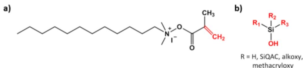
**Figure 2.** a) Quaternary ammonium methacrylate based monomer with reactive double bond ready for free radical polymerization, b) Anchoring units of silane after hydrolysis ready for further condensation reaction.
