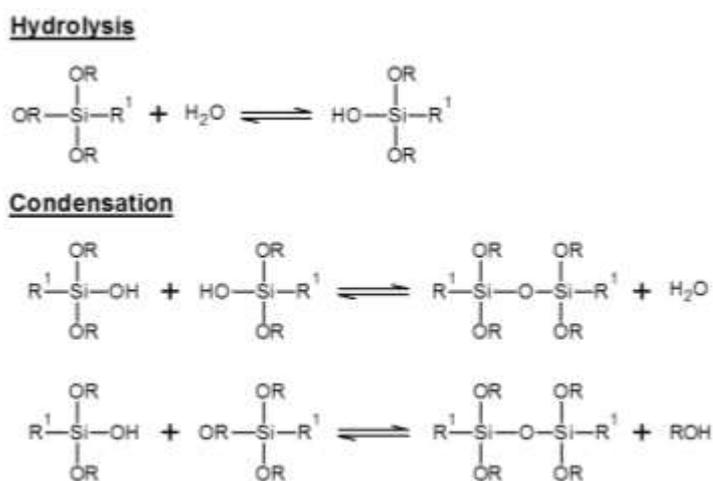
**Figure 3.** Representation of the reactions that take place during the sol–gel process.
