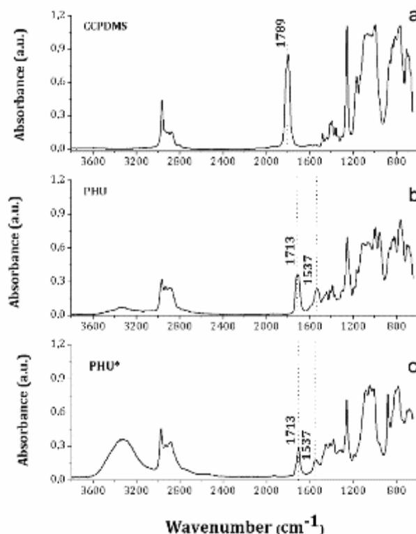
**Figure 3. FTIR-ATR spectra: a) CCPDMS; b) PHU and c) PHU\* polymer solutions.**
