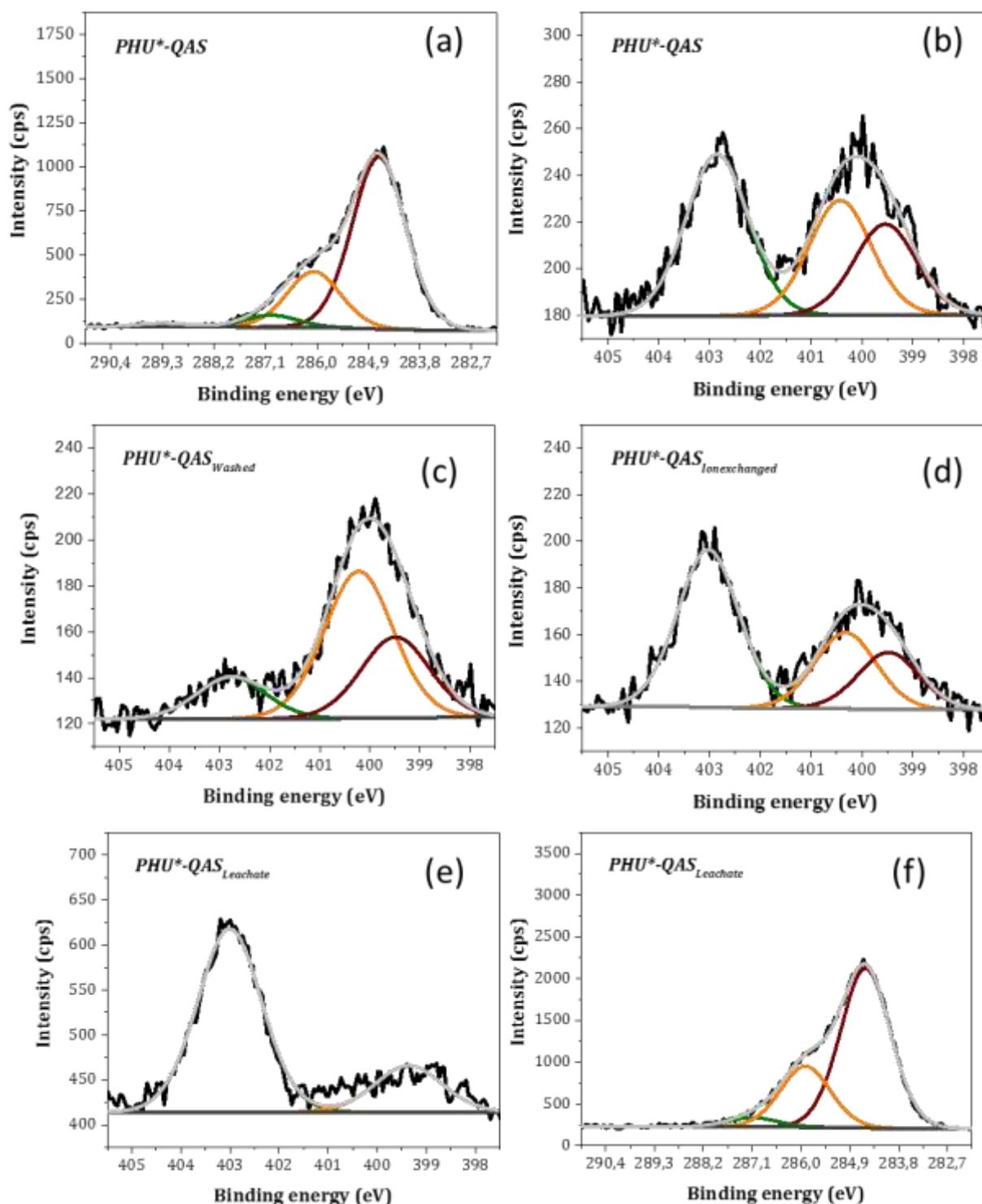
**Figure 6.** XPS narrow scans obtained for: **a)** C<sub>1s</sub> for PHU\*QAS coating; **b)** C<sub>1s</sub> of PHU\*QAS leachate solution; **c)** N<sub>1s</sub> for PHU\*QAS coating; **d)** N<sub>1s</sub> for PHU\*QAS washed coating; **e)** N<sub>1s</sub> for PHU\*QAS ion exchanged coating and **f)** N<sub>1s</sub> of PHU\*QAS leachate solution.
