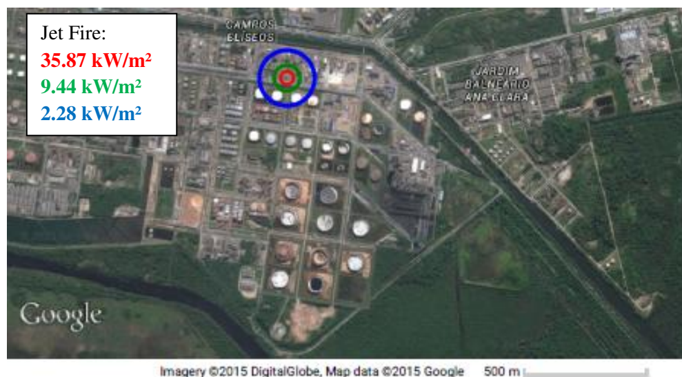
Figure 39. Jet fire radiation flux after a supposed accident in the natural gas unit of a refinery according to the distance from the receiver. Vulnerable area affected by the jet is represented according to the distance from the receiver. (GOOGLE MAPS, 2015)
