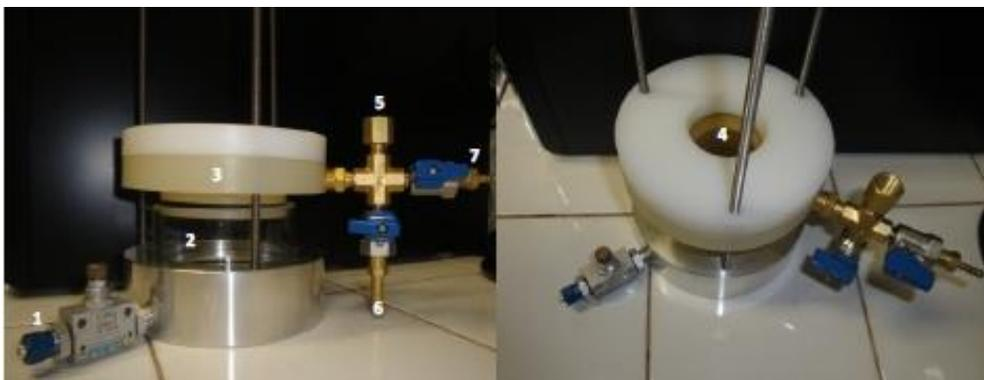
**Figura 5.2.** Reator *laser cracking*.
