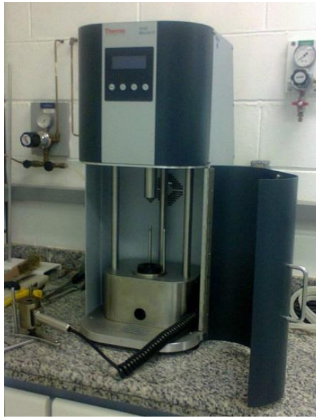
Figura 12. Mini-injetora Thermo Scientific , HAAKE Minijet II .
