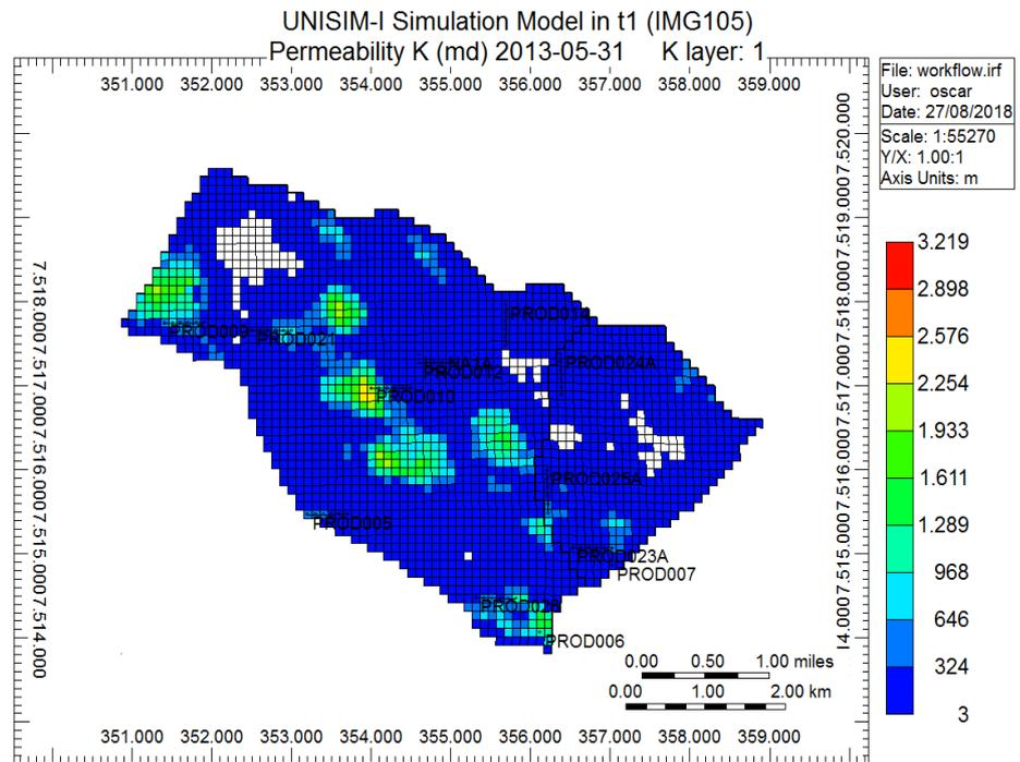
**Figure 5.11: Distribution of Permeability in K direction. UNISIM-I-D (RM9-img105)**
