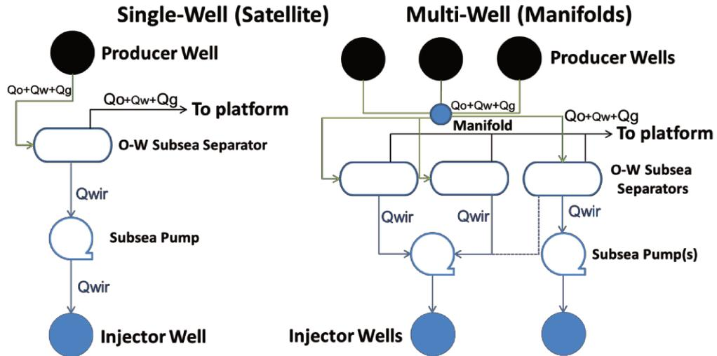
Figure 4.3: Differences between single-well and multi-well arrangements
