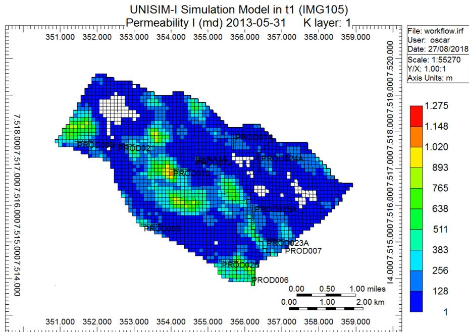
Figure 5.9: Distribution of Permeability in I direction. UNISIM-I-D (RM9-img105)
