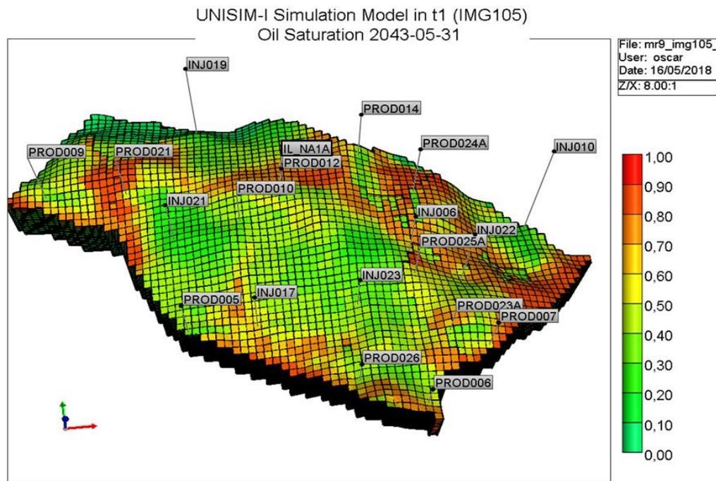
Figure 5.2: Oil Saturation Distribution in case UNISIM-I-D. Time 10957
