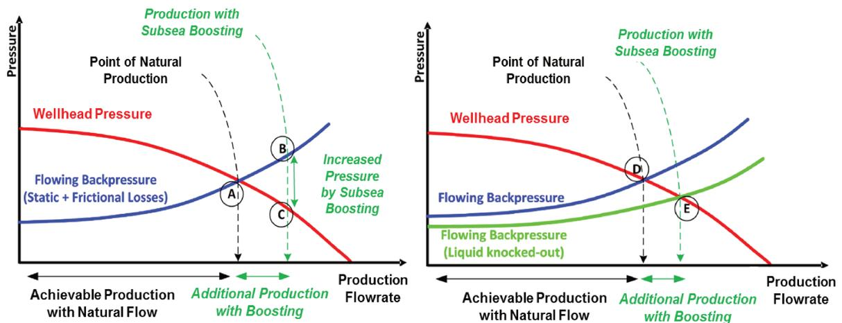
Figure 2.2: Incremental recovery due to the implementation of subsea processing (Sandy and Hasan, 2016)
