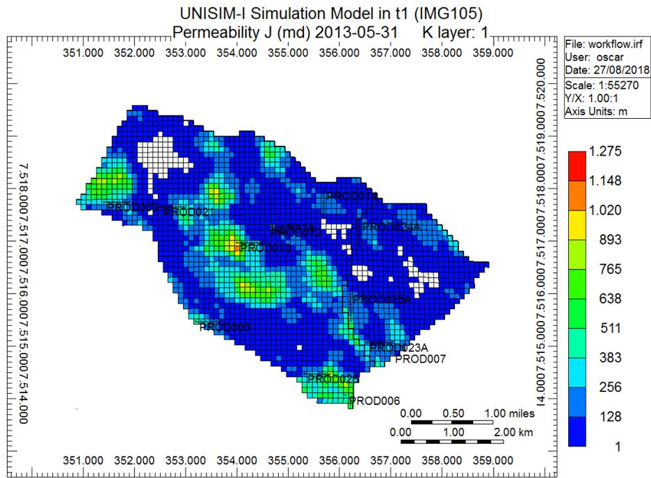
**Figure 5.10: Distribution of Permeability in J direction. UNISIM-I-D (RM9-img105)**
