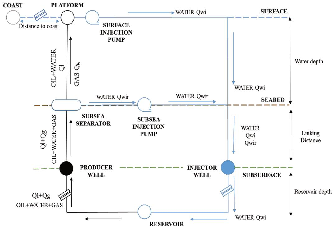
**Figure 4.4: Production network for a single-well implementation of O-W subsea separation and PWRI**
