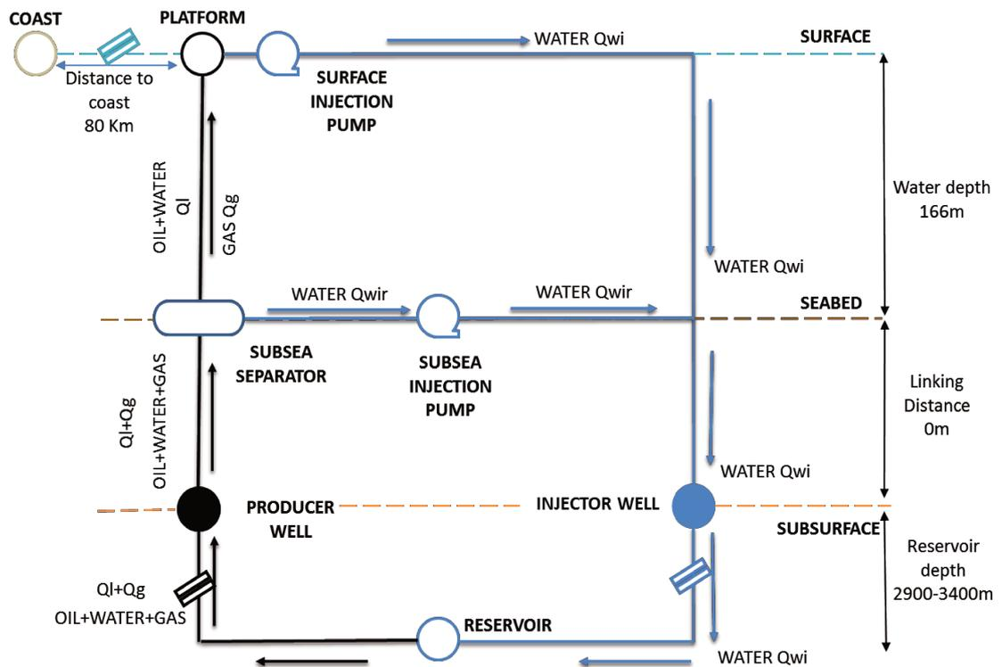
Figure 5.13: Final production network for single-well application
