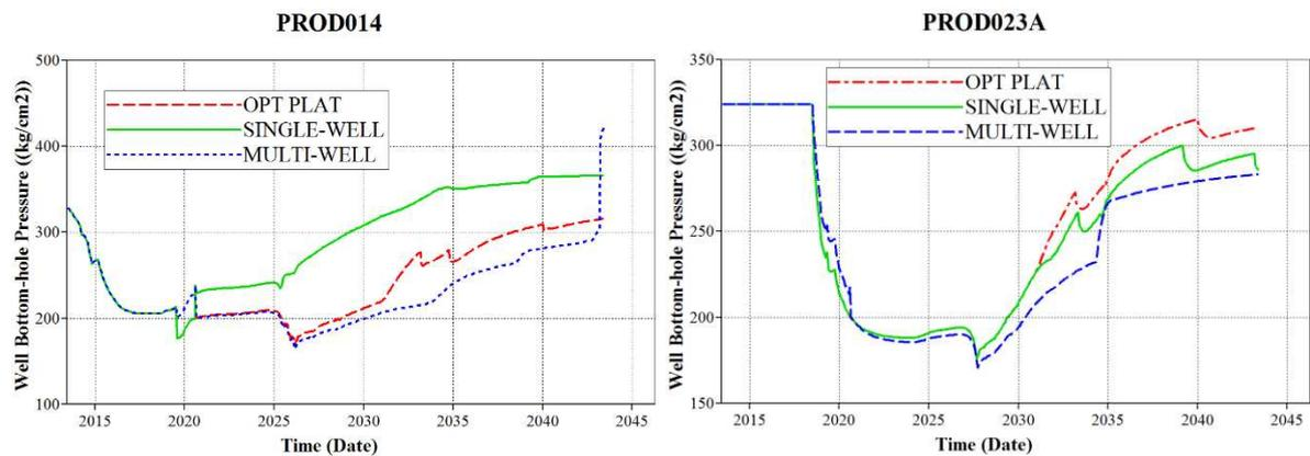
**Figure 6.14: BHP of producers PROD014 and PROD023A**
