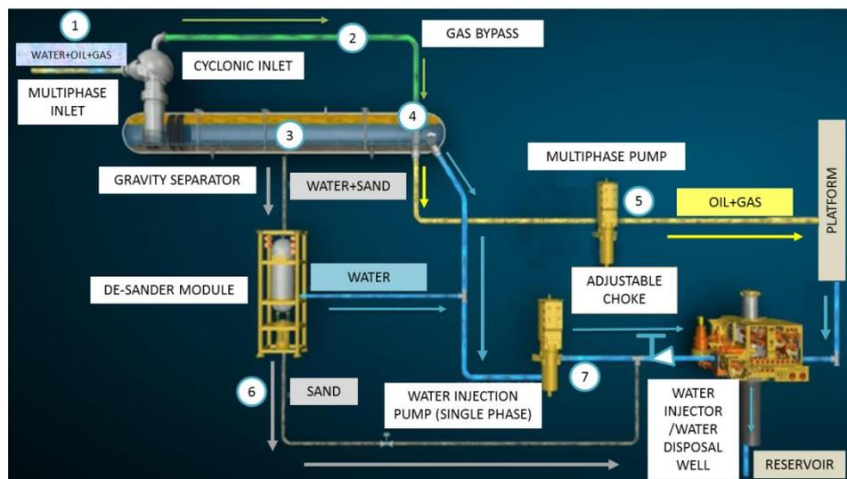
Figure 2.3: Subsea separation and water re-injection process (Modified from Hendricks et al., 2016)
