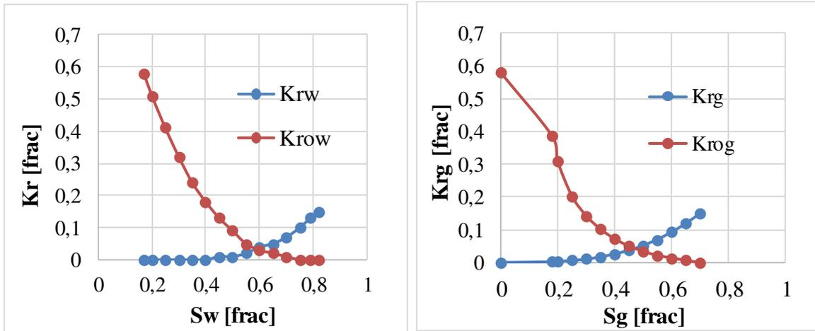
Figure 5.12: Relative permeability curves ( $K_r$  and  $K_{rg}$ , respectively) used in RM9, UNISIM-I-D
