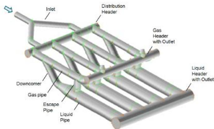
Figure 2.4: Schematic representation of multipipe separators (Hannisdal et al., 2012)
