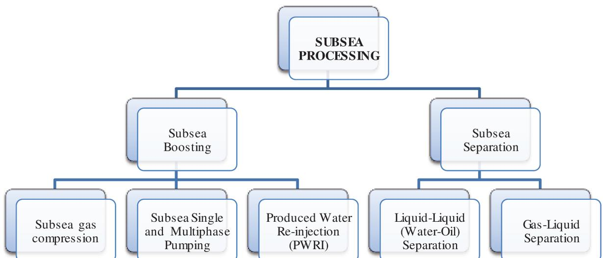
Figure 2.1: Main components of subsea processing (Modified from Karra et al., 2010)
