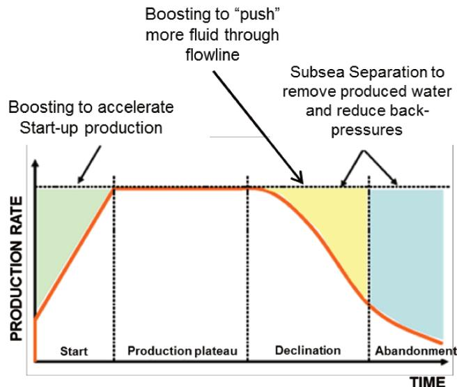
Figure 3.2: Applications of subsea processing at different production stages of a field (Modified from Lim and Gruehagen, 2009)
