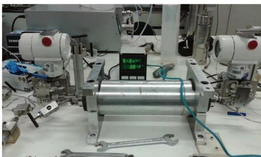
a) *Core holder* utilizado
