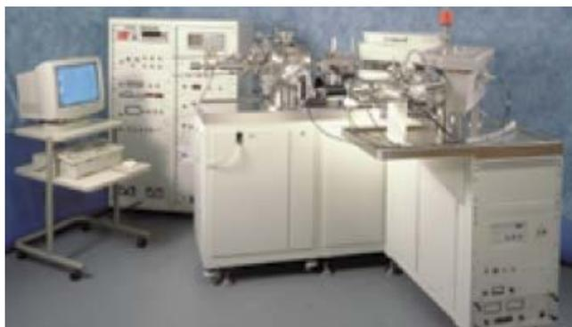
Figura 4.28 – Equipamento VG 9000 da Thermo Electron de GDMS (Glow Discharge Mass Spectrometry). [Thermo Electron, 2009]
