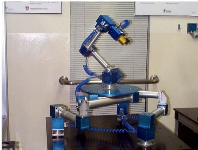
**Figura 4: Manipulador híbrido (ROBOTICS RESEARCH CENTER, NANYANG TECHNOLOGICAL UNIVERSITY).**
