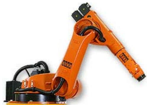
(b) Manipulador Serial KR-3 KS (KUKA robot Group)
