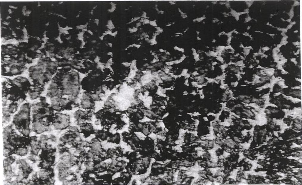
**Fig. 10.25 - Micrografia - camada - P20 (2) (0.1 g/s) - 2000 x**
