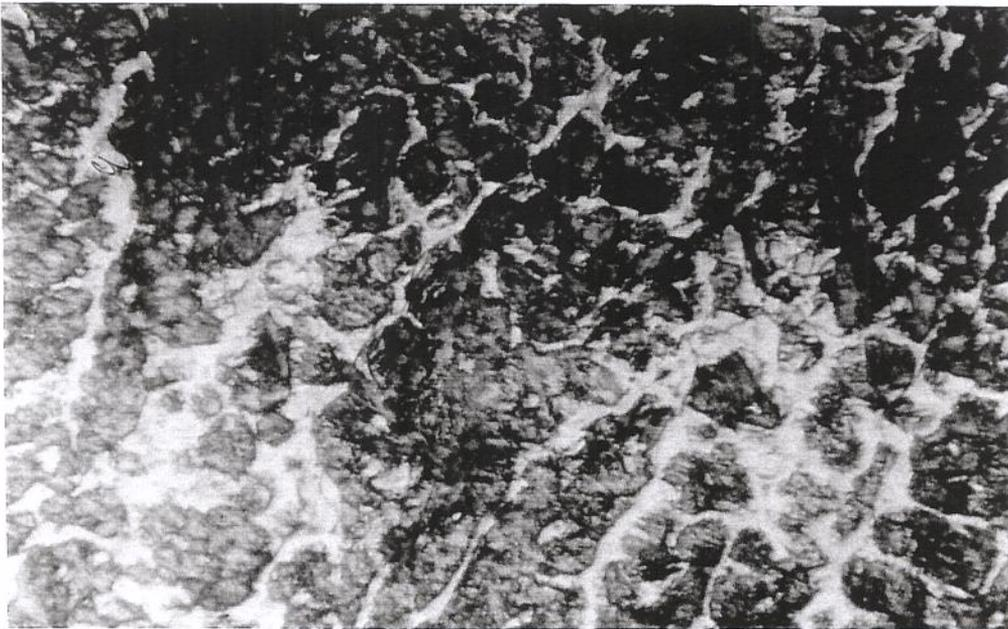
**Fig. 10.23 - Micrografia - camada - P20 (2) (0.1 g/s) - 2000 x**
