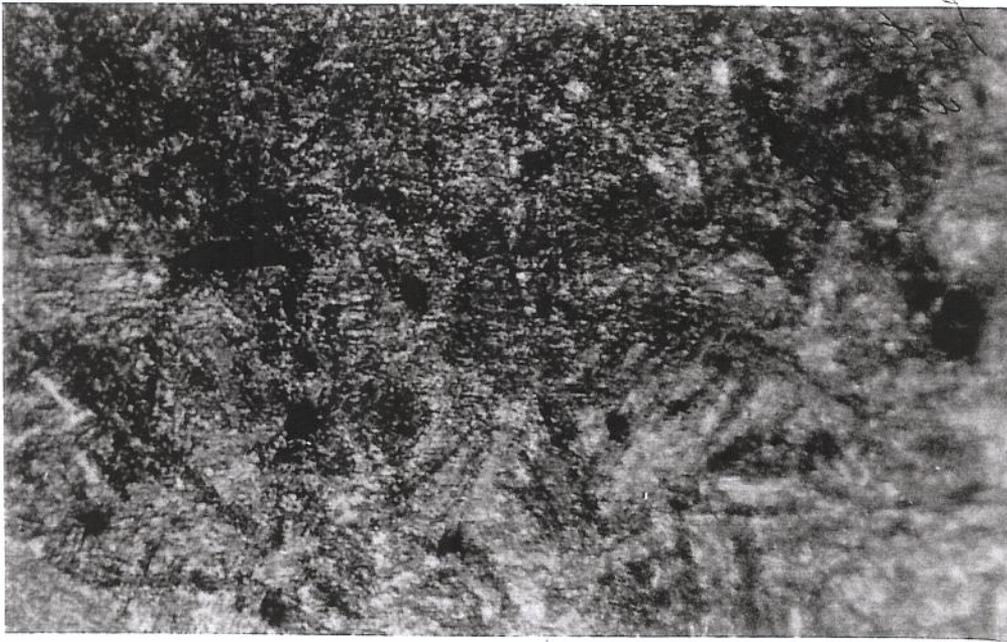
**Fig. 10.28 - Micrografia - interface substrato - ZTA - P20 (2) (0.15 g/s)- 2000 x**
