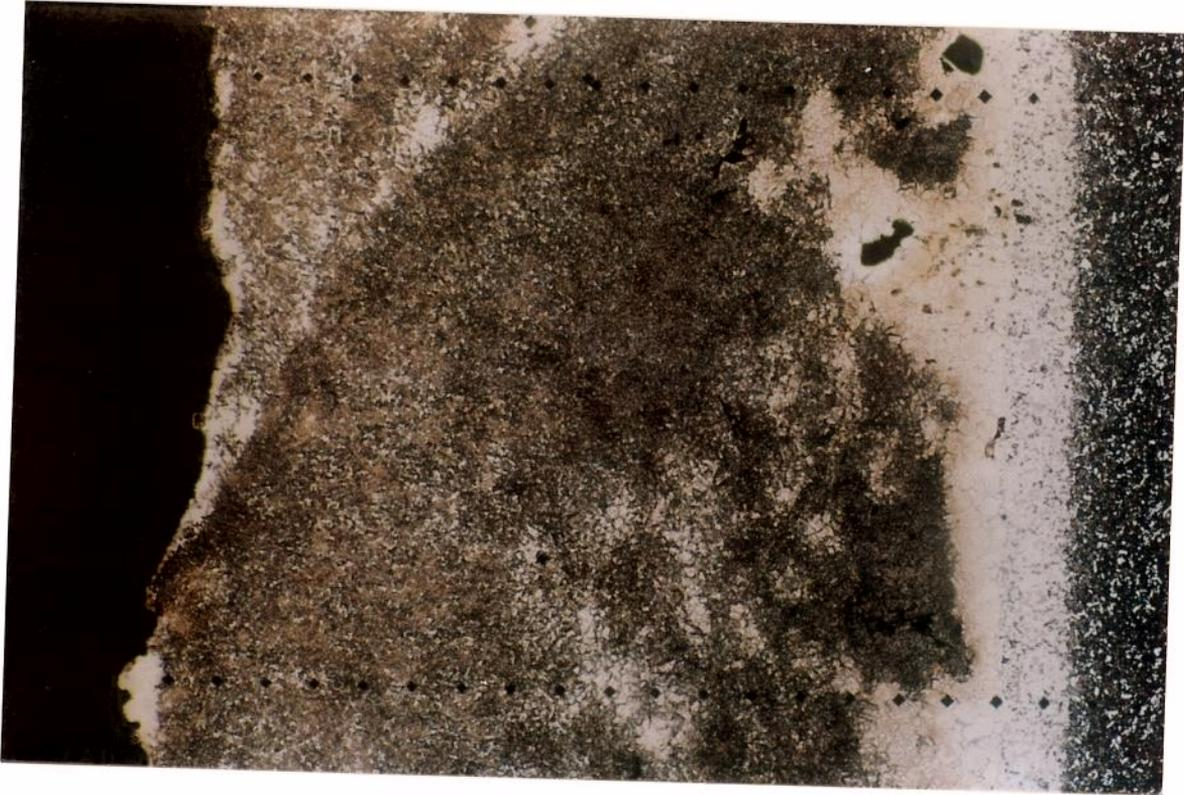
**Fig. 10.40 - Micrografia - camada - 2<sup>a</sup> exper. P20 (2) (0.15 g/s) - 125 x**
