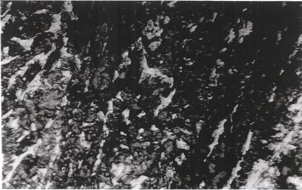
**Fig. 10.22 - Micrografia - camada - P20 (2) (0.1 g/s) - 2000 x**
