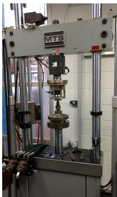
Figure 67 – Sample under compressive load in MTS testing machine.
