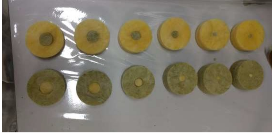
Figure 27 – Samples with mesopores filled: glasswool substrate filled with rockwool (above) and rockwool substrate filled with glasswool (below).
