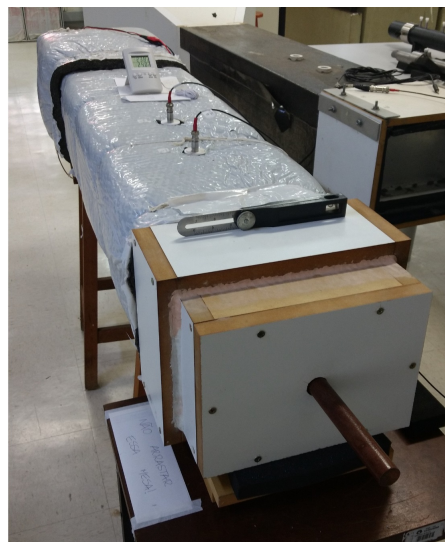
Figure 24 – Sound absorption test using the impedance tube of rectangular cross section.
