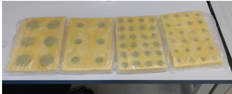
Figure 36 – Glasswool substrate samples with mesopores filled with rockwool.
