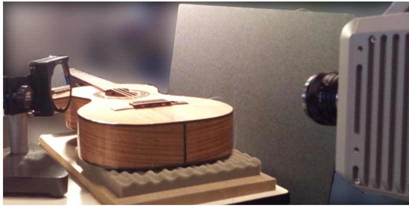
Figure 4.2: Experimental setup for motion analysis of the viola caipira strings using a high speed camera.
