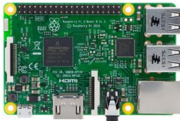
Figura 5.5 – Raspberry Pi 3 - Fonte: Raspberry Corporation.
