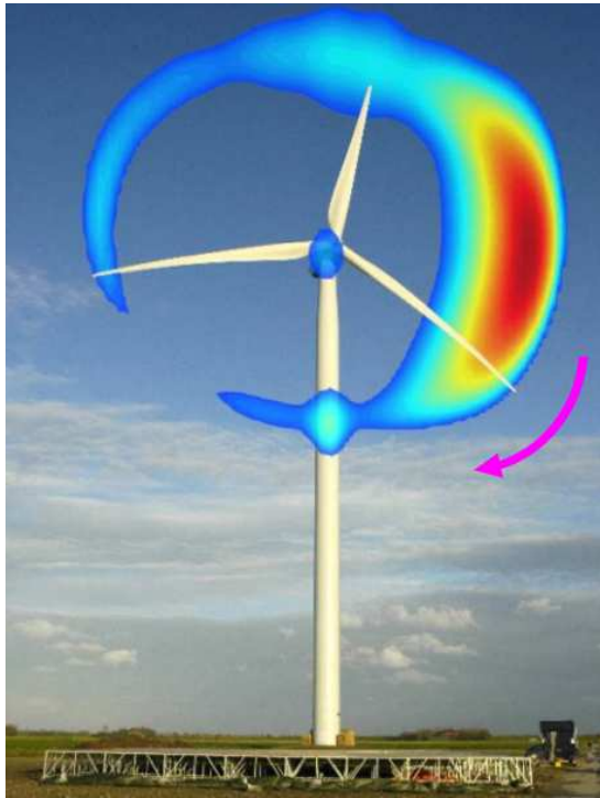
(a) Main sources of wind turbine noise.
