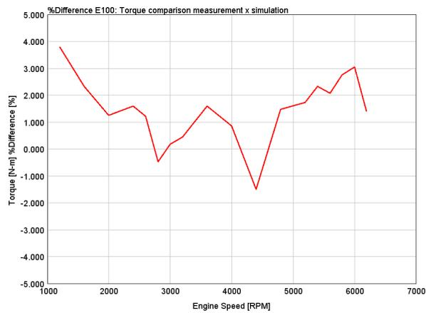
(c) Error difference - engine torque.
