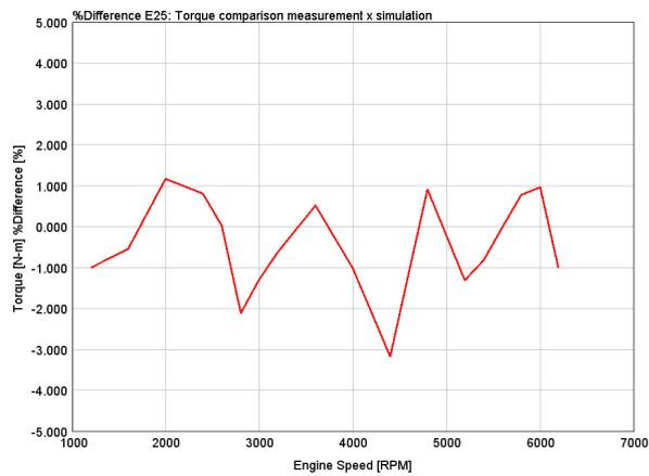
(c) Error difference - engine torque.
