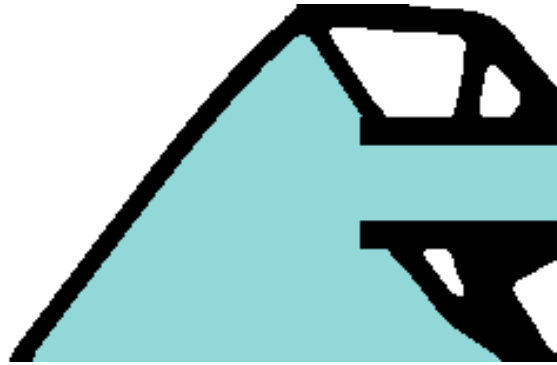
Figure 5.22: Structural topology solution for the flow chamber example.
