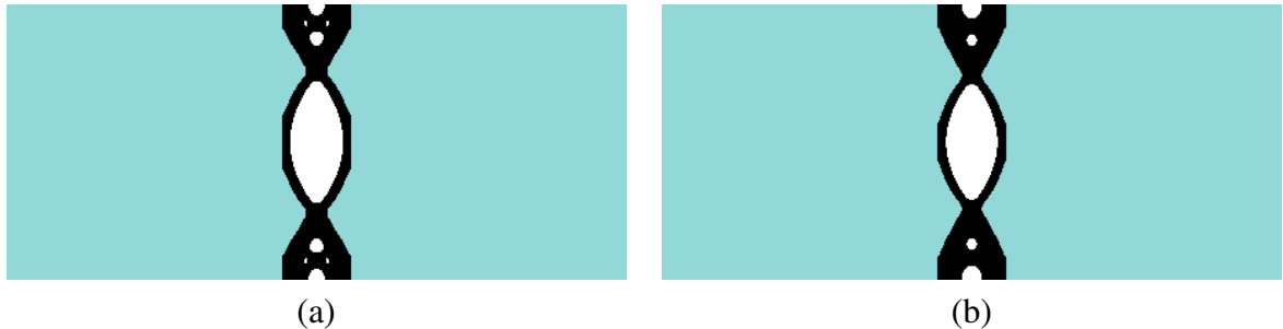
Figure 4.3: Clamped beam solutions obtained with the BESO method with initial structure starting from the: (a) full design domain; (b) initial guess design with 50% of the design domain.
