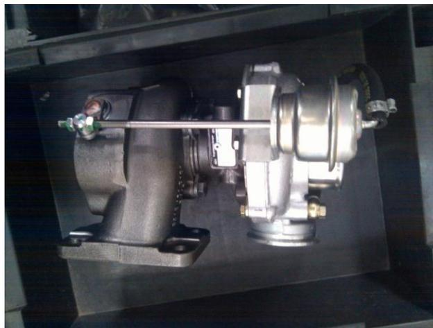
Figura 24: Turbocompressor BorgWarner
