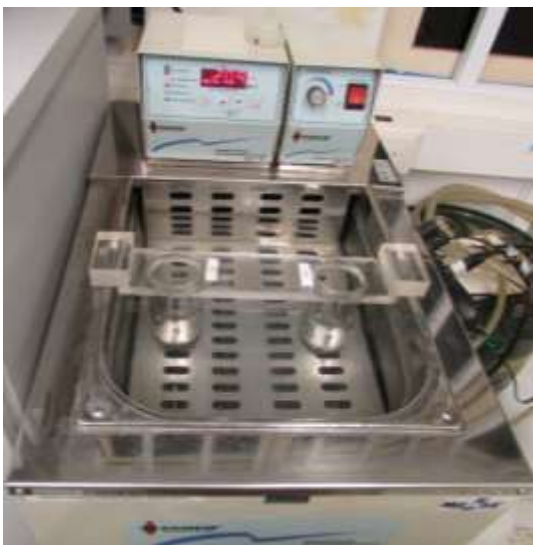
Figure 8. Test jar carrying apparatus in a thermostatic bath at 21 °C for pour point determination.
