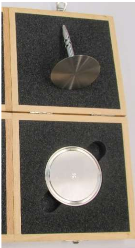
Figure 12. Cone-plate geometry with cone size of 60 mm.
