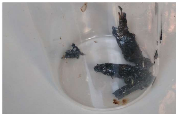
Figure 12. Wax deposit removed in the pig operation.
